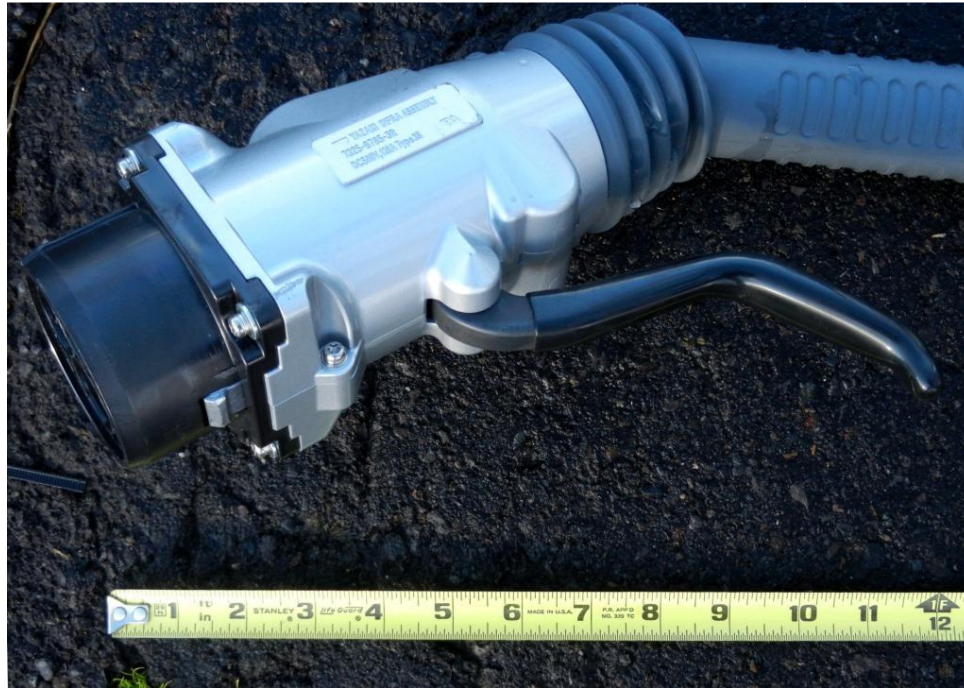
FIGURE 13: SIZE OF DC FAST CHARGER CONNECTOR
